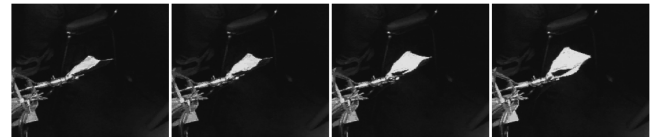
Fig. 2 Results of an experimental demonstration of the clap–fling phenomenon with a sequence of still captures of wing set on test apparatus using a strobe light.
